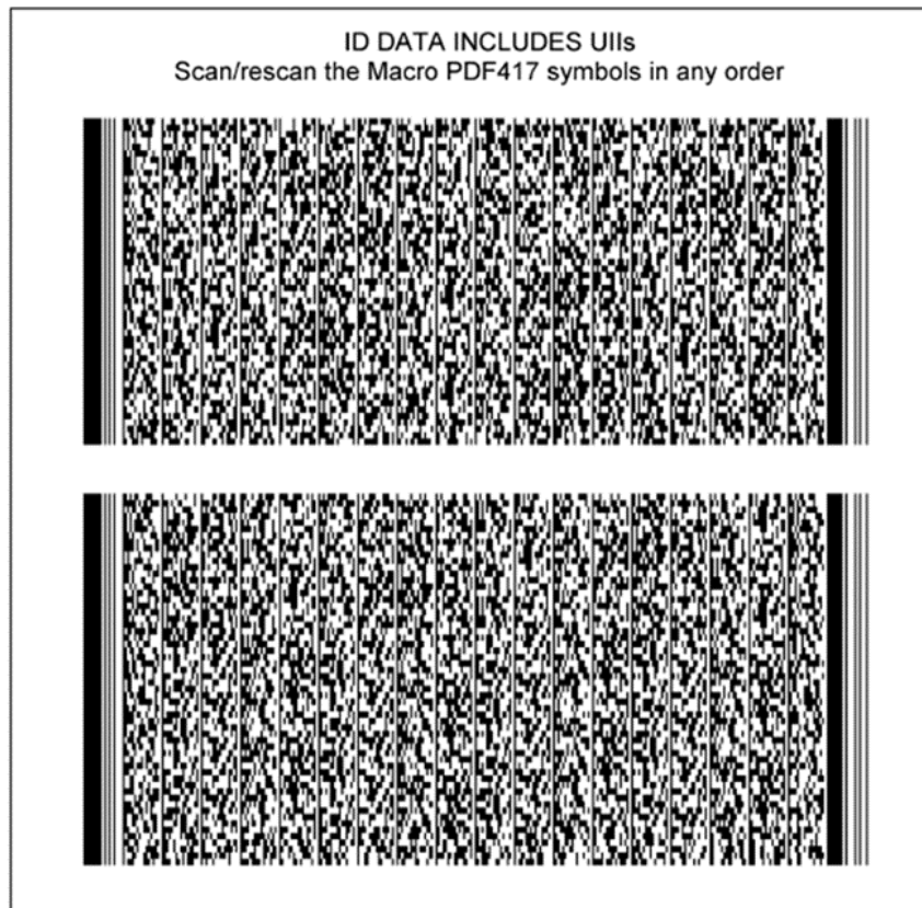
NOTE: Example is actual size and can be used for scanner testing. FIGURE 20. Macro PDF417 bar codes on exterior container label.
